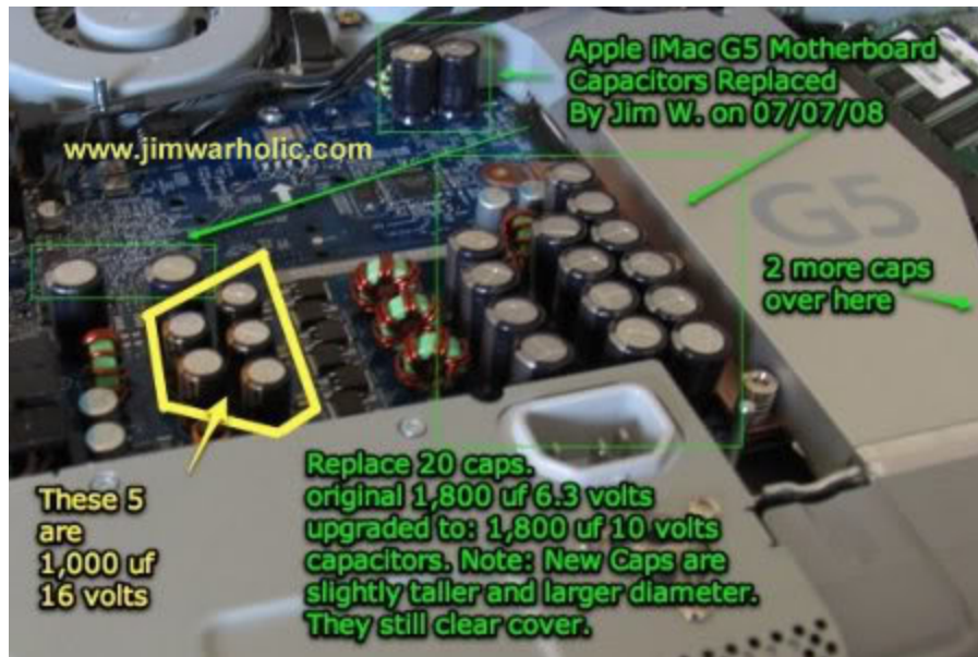
Location of Capacitors on MOB Next to Power Supply on 1st Generation Apple iMac G5
